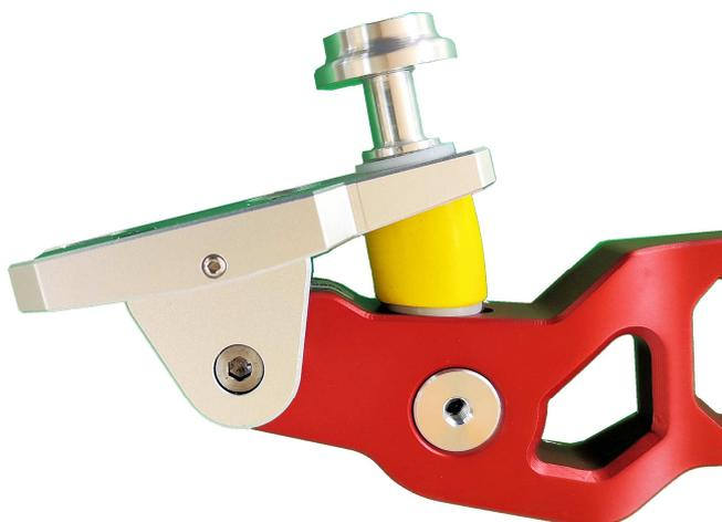
Pockets of the limbs are set at factory at minimum poundage position. +9 turns of the bolts will move the pockets to the neutral position corresponding to 15% angle of their upper surface and -3 turns from maximum poundage. (total excursion, +12 turns in full safety).
