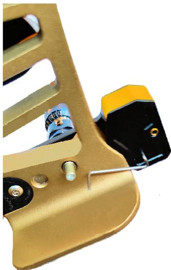
Rest has to be assembled to the bow by the use of the 5/16-24 screw and M8 washer provided, fixing to the front 5/16 tapped hole in the riser. Main part of the body of the rest should never touch the body of the riser. 1 mm minimum air should exist between the two parts.
