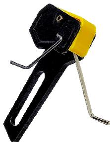
Cover has to be re-assembled engaging its lower part first and after pushing the top part until it "clicks" on the body of the rest.
